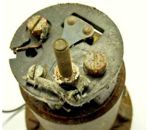
3. Rotate up the pedestal and remove the brass terminal post.
