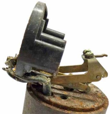
4. Return pedestal, pull the electrical wires away as far as possible and turn pedestal anti-clockwise, note how many turns are required until points are free of the shaft (mine took 8 full turns).
