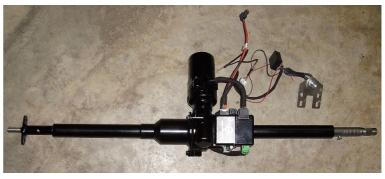
complete column to replace the factory column depending on make and model. The ECU is part of the motor
