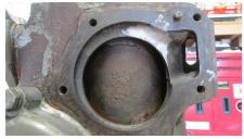
Have just ground away the step on the block casting, where the water-pump is fitted, to improve the water flow and improved the entry channel into the side water gallery. These modifications have been recommended in previous MGC articles and endorsed by the well-respected and much-loved UK MGC Register technical advisor Vic Young and Bruce Ibbotson. Will let you know how we get on. Photo taken after grinding away the webbing in the hole on the right.
